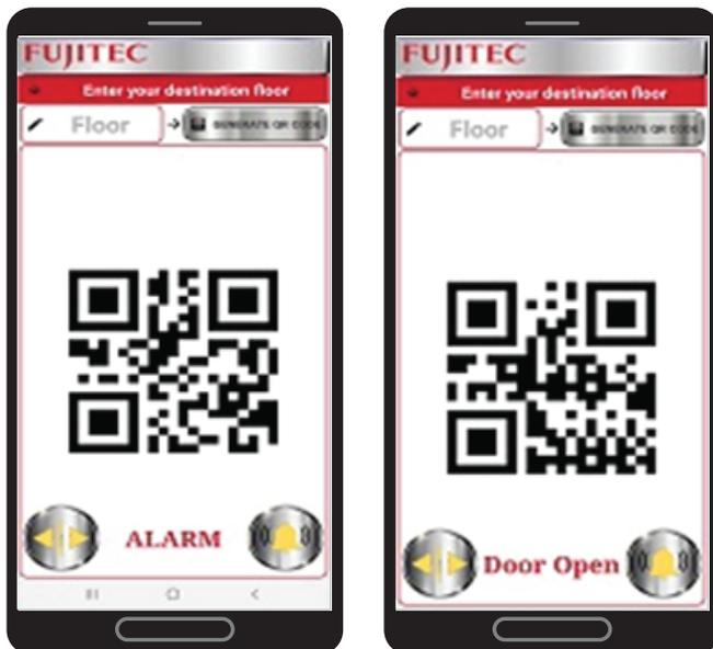
The Touchless Module can be connected with the existing COB module and configured based on the number of floors and number of elevators. The system will detect the QR code through microcomputer with help of camera and will communicate the required floor registration.
